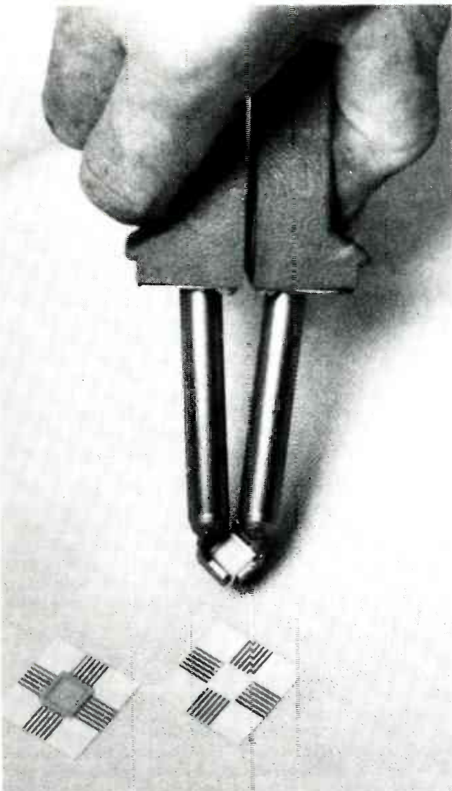
FIG. 10—A PAK-X-TRAC™ DESOLDERING SCISSORS can be used to simultaneously heat the terminals on all four sides of a quad PLCC.
