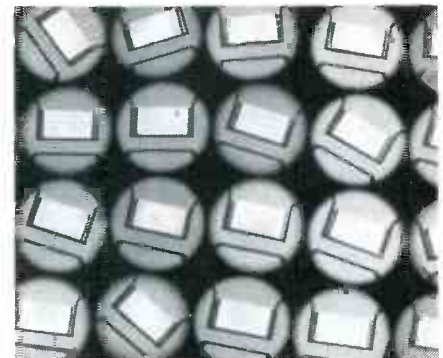
FIG. 5—AN X-RAY PHOTO SHOWS some transistor-cells that are poorly bonded to the die, which will result in hot-spots.
